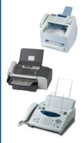
**LASER TECHNOLOGY** Fax machines based on laser technology produce excellent quality text and graphics and typically have a lower cost per page than other print technologies, particularly laser models with high-yield toner and drum combos. Laser fax machines are best suited for mid- to large-size offices where a wider range of high-performance features are required.
